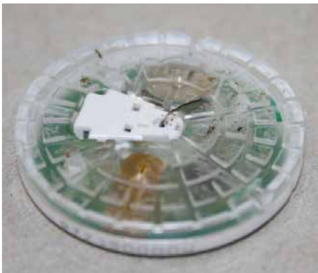
Figure 3: Used freestyle sensor showing the sensing electrode that sits in the interstitial space.
